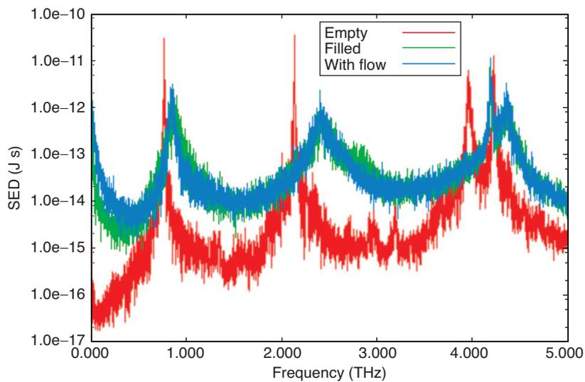
Figure 3. Frequency dependent SED plot (along  $K_z = 0$ ) showing the four acoustic modes for (8,8) CNT
