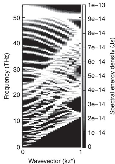
Figure 1. SED Profile for Empty (8, 8) CNT
