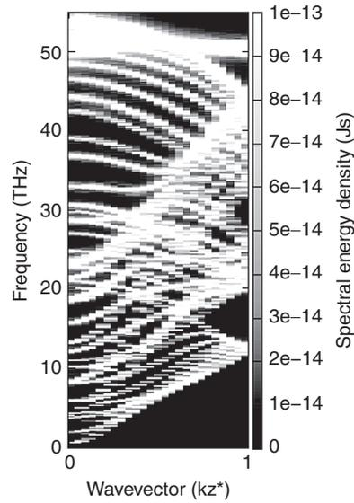
Figure 2. SED profile for filled (8, 8) CNT
