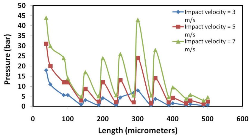
Figure 8(a): Variation of pressure with distance from point of impact, with multiple velocities. The fraction of solid in contact = 0.37
