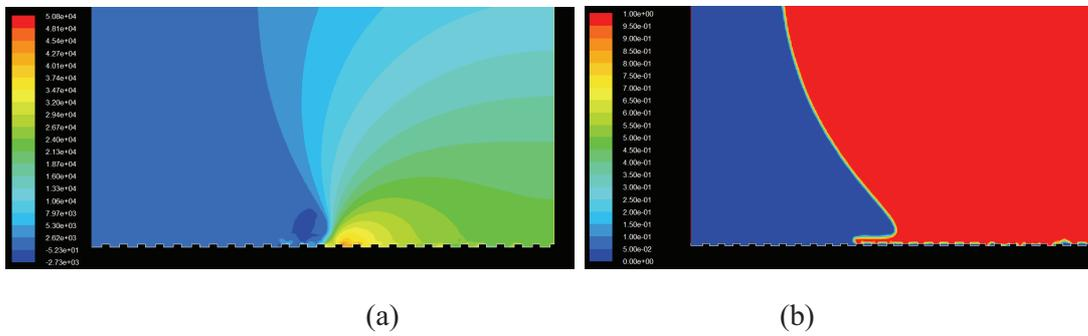
Figure 6: Contour corresponding to late regime, water hammer pressure is not dominant, for an impact velocity of 3 m/s. (a) Pressure contour (Pressure in Pa) (b) Phase contour
