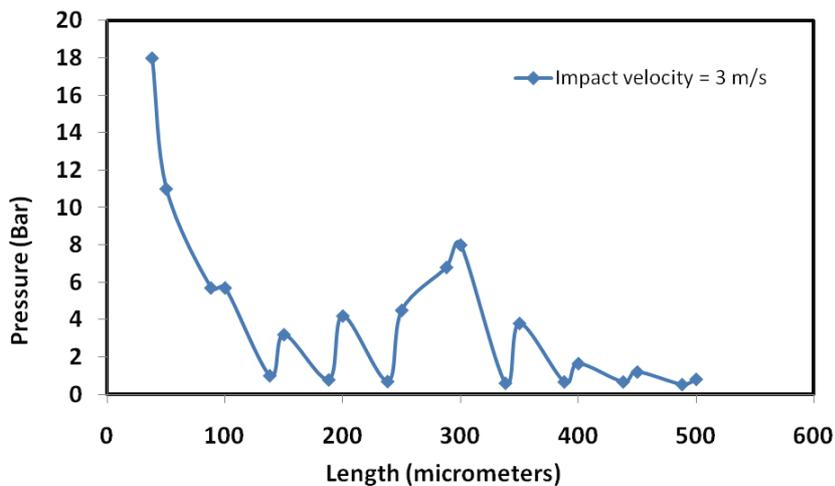
Figure 7. Variation of pressure with distance from point of impact. The fraction of solid in contact = 0.37
