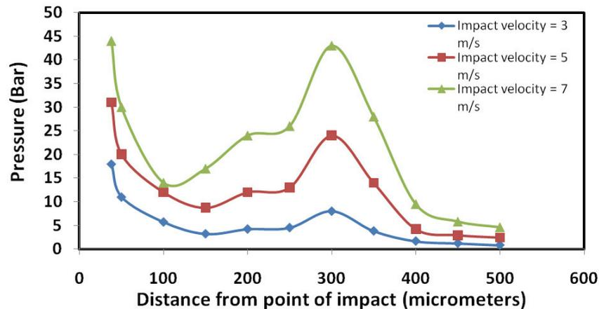
Figure 8(b). Variation of pressure with distance from point of impact with multiple velocities (only water hammer pressure) (The fraction of solid in contact = 0.37)
