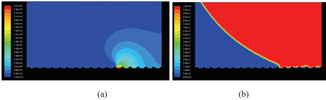
Figure 5. Contour corresponding to early regime, dominated by water hammer pressure, for an impact velocity of 3 m/s (a) Pressure contour (Pressure in Pa) (b) Phase contour
