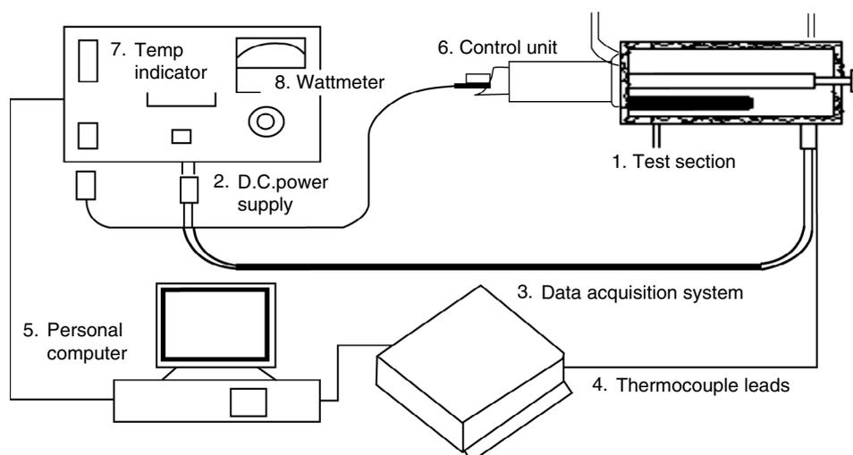
Figure 1a. Schematic representation of the experimental set up.
