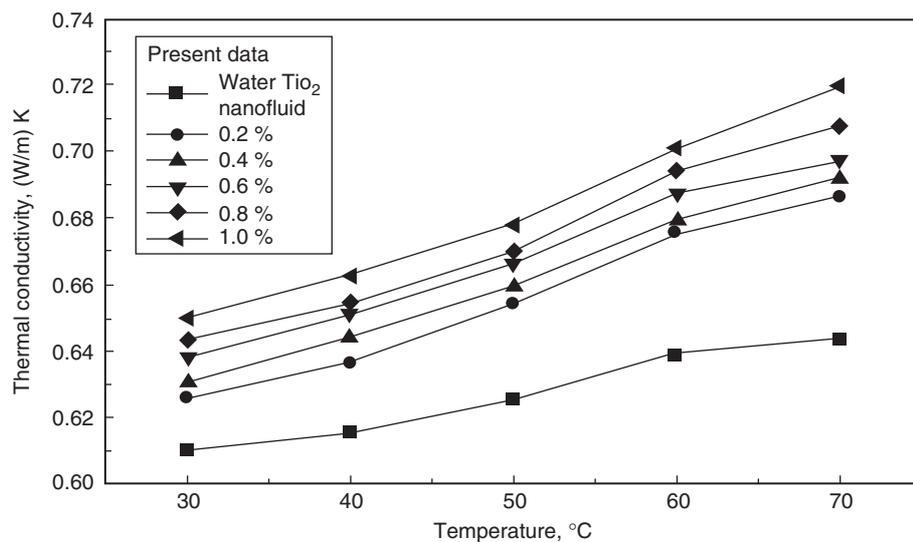
Figure 3. Thermal conductivity of TiO<sub>2</sub>-water nanofluids as a function of temperature and volume concentration.
