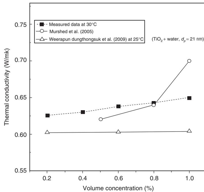
Figure 6. Comparison of the measured thermal conductivity at room temperature with those reported by various researchers.
