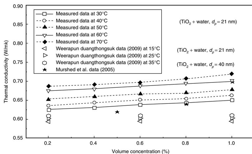
Figure 5. Comparison of the measured thermal conductivity enhancement with those obtained various researchers.
