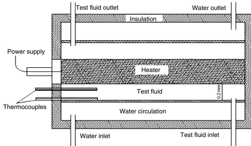
Figure 1b. Details of the test section.
