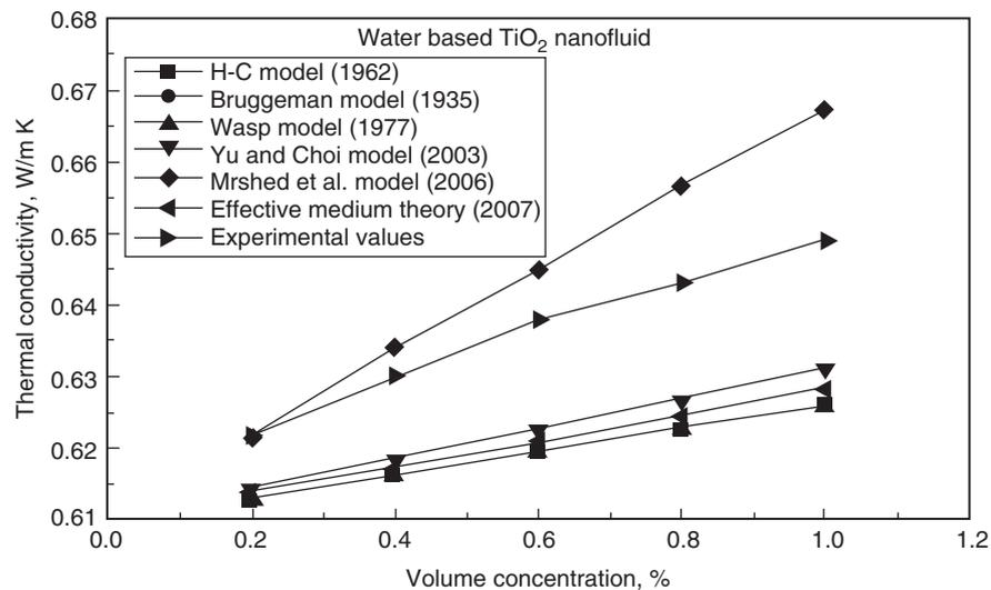
Figure 4. Comparison of measured thermal conductivities with those obtained from various correlations.
