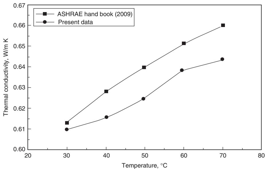
Figure 2. Comparison of the measured thermal conductivity with reference data.
