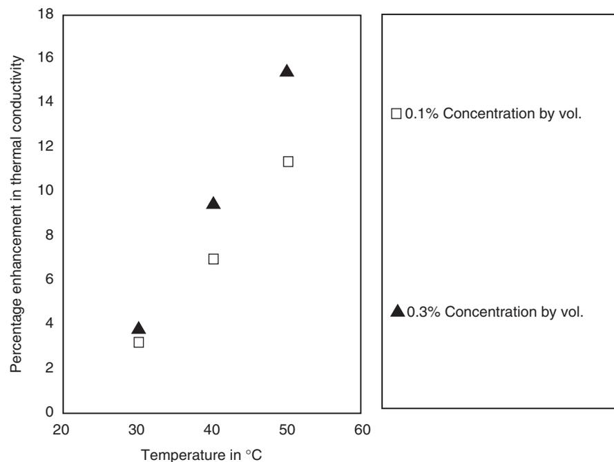
Figure 1. Enhancement in the thermal conductivity of ATF-TiO<sub>2</sub> nanofluid as a function of temperature.
