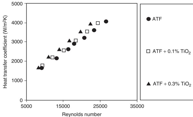
Figure 5. Convective heat transfer coefficient of ATF-TiO<sub>2</sub> nanofluid as a function of Reynolds number.
