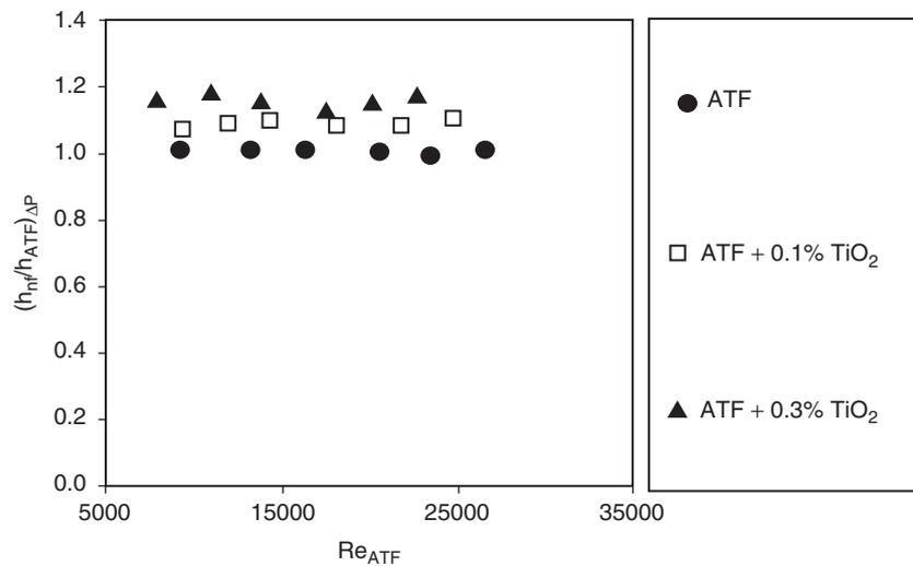
Figure 7. Ratio of heat transfer coefficient of ATF-TiO<sub>2</sub> nanofluid to that of ATF as a function of Reynolds number.
