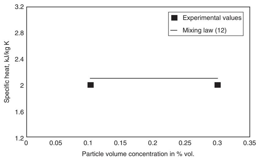
Figure 4. Specific heat of ATF-TiO<sub>2</sub> nanofluid as a function of particle volume concentration.
