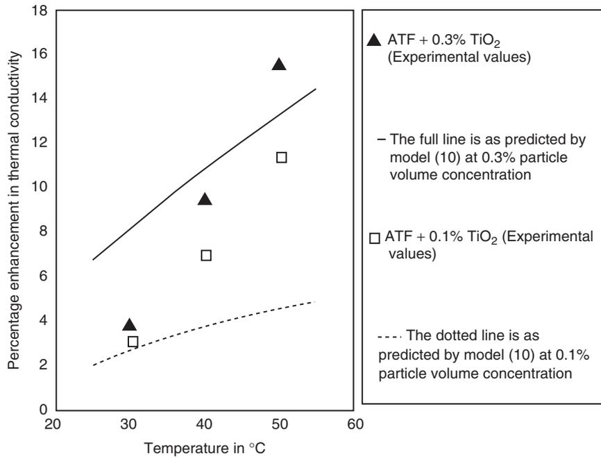
Figure 2. Comparison of measured enhancement in thermal conductivity of nanofluid with that predicted using a model by Prasher et al. [10].
