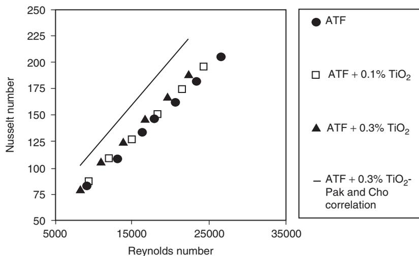
Figure 6. Nusselt number of ATF-TiO<sub>2</sub> nanofluid as a function of Reynolds number.
