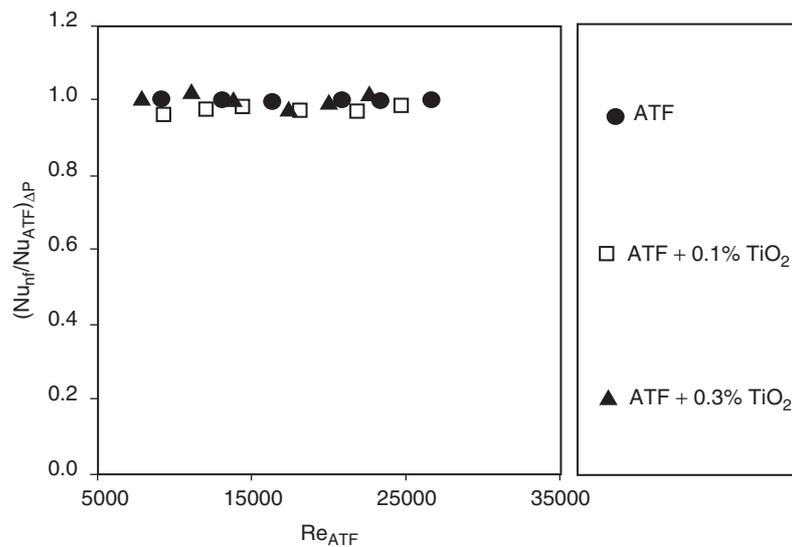
Figure 8. Ratio of Nusselt number of ATF-TiO<sub>2</sub> nanofluid to that of ATF as a function of Reynolds number.
