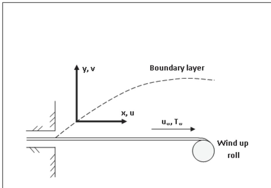
Figure 1 Flow Model and Coordinate System
