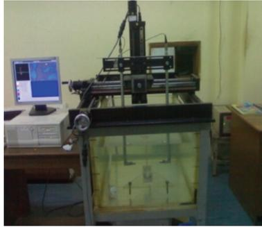
Figure 2. Ultrasonic through transmission scanning set up
