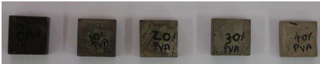
Figure 8. Bulk adhesive samples prepared to measure velocity and density variation
