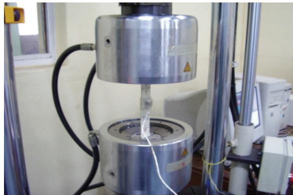
Figure 16. Test set up for determining the bond strength.
