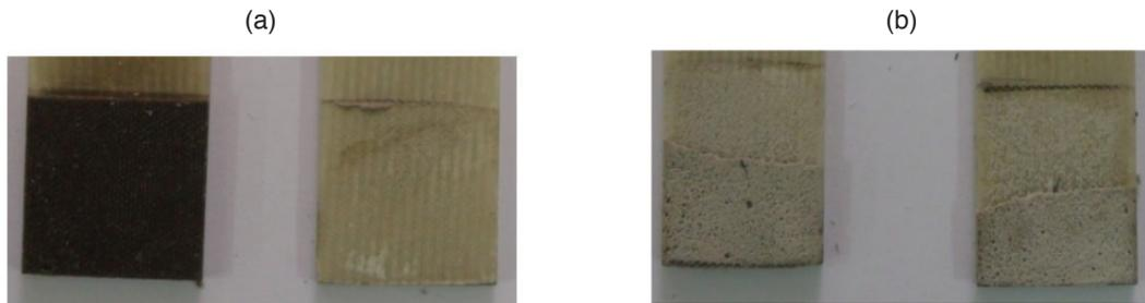
Figure 18. Failed Adhesive joints of a) Healthy Sample and b) PVA added sample.
