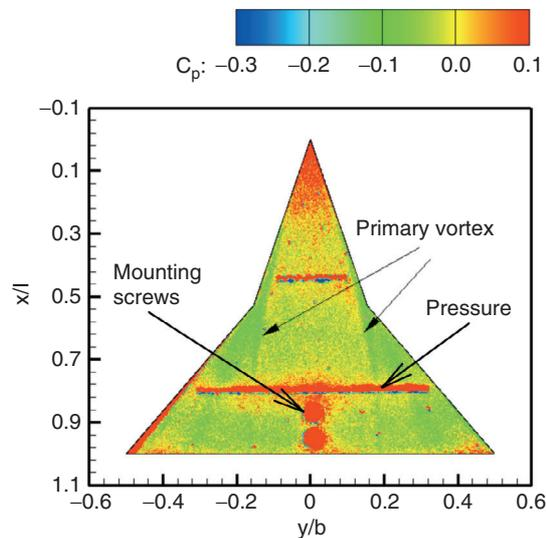
Figure 5.  $C_p$  distribution over delta wing at  $0^\circ$ .
