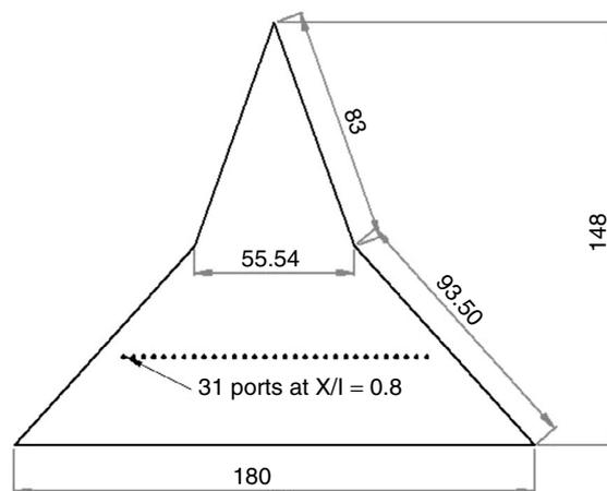
Figure 2. Dimensions of the Model in mm.
