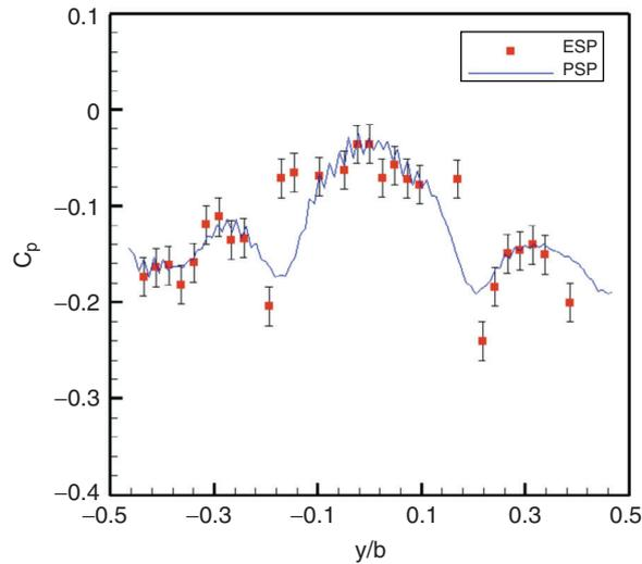
Figure 9. Comparison between ESP and PSP measurement at 5°.
