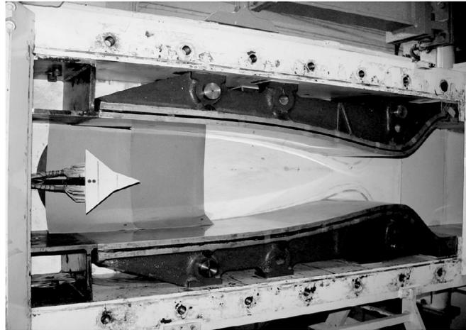
Figure 1. Photograph of model mounted in the 0.3 m Trisonic Tunnel.
