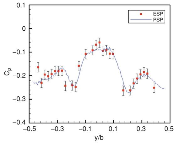
Figure 12. Comparison between ESP and PSP measurement at 10°.
