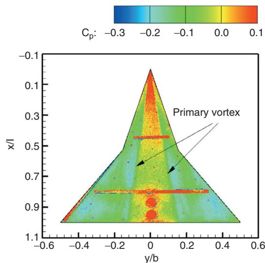
Figure 8.  $C_p$  distribution over delta wing at  $5^\circ$ .
