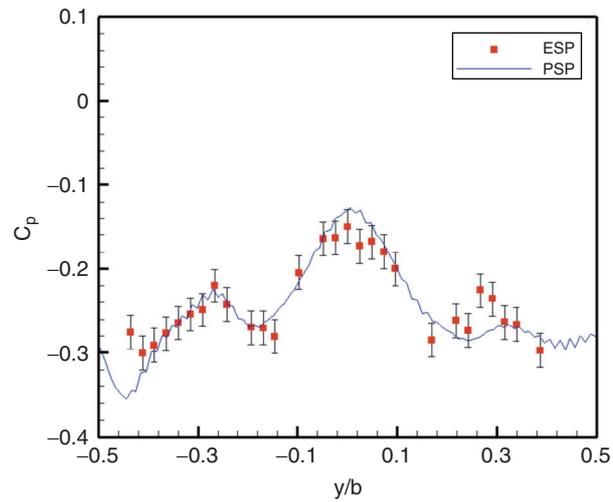
Figure 15. Comparison between ESP and PSP measurement at  $15^\circ$ .
