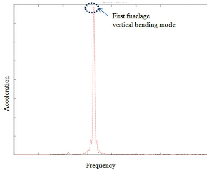
Figure 14. Vertical Acceleration with Frequency at Nose tip for MSR case
