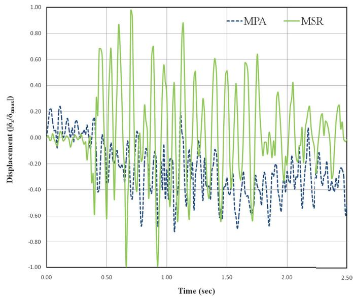
Figure 7. Lateral Displacement response at Fin tip location
