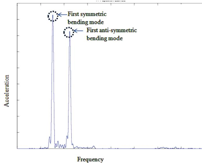
Figure 15. Vertical Acceleration with Frequency at Wing tip for MSR case
