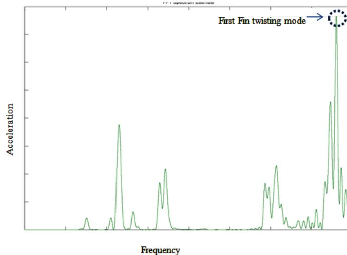
Figure 13. Lateral Acceleration with Frequency at Fin tip for MSR case
