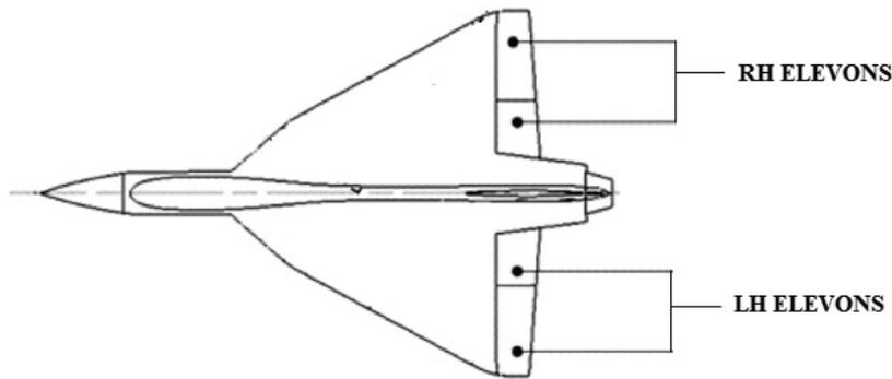
Figure 1. Typical Tailless Delta Wing Aircraft with ELEVONS
