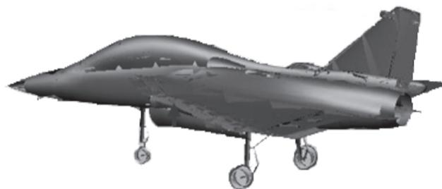
Figure 2. Typical MBS model showing Main landing gear and Nose landing gear
