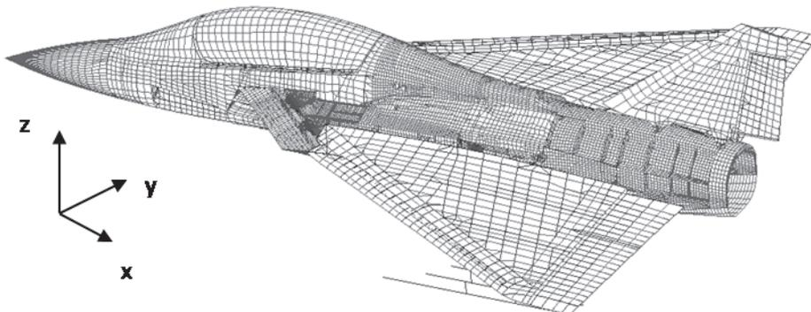
Figure 4. Finite Element Mesh model using MSC Nastran
