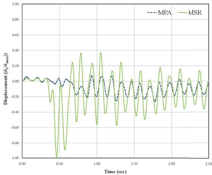
Figure 9. Vertical Displacement response at Wing tip location
