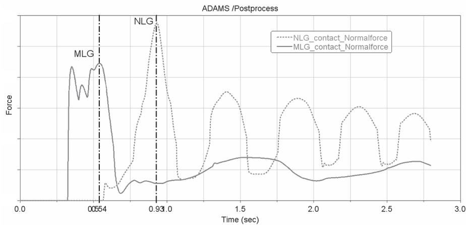
Figure 3. Landing simulation showing force response plot for Main landing gear and Nose landing gear using MSC Adams
