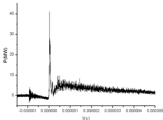
Figure 1. The laser1 pulse waveform
