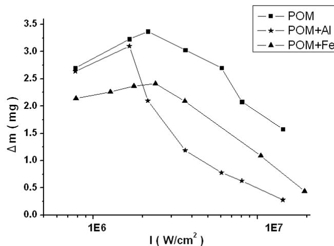
Figure 4. Mass loss per pulse versus laser power density for three kinds of propellants
