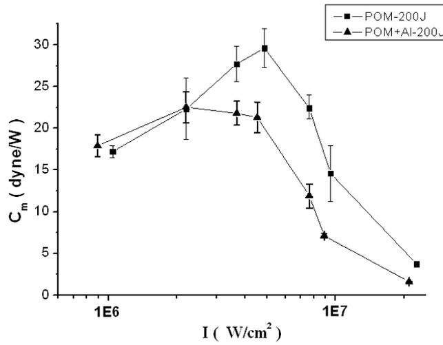
Figure 8. Experimental  $C_m$  versus laser power density curves for laser 2
