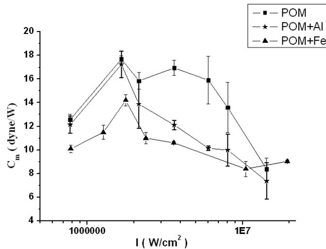
Figure 3. Experimental  $C_m$  versus laser power density curves for three kinds of propellants
