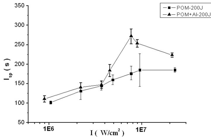
Figure 9. Experimental  $I_{sp}$  versus laser power density curves for laser 2
