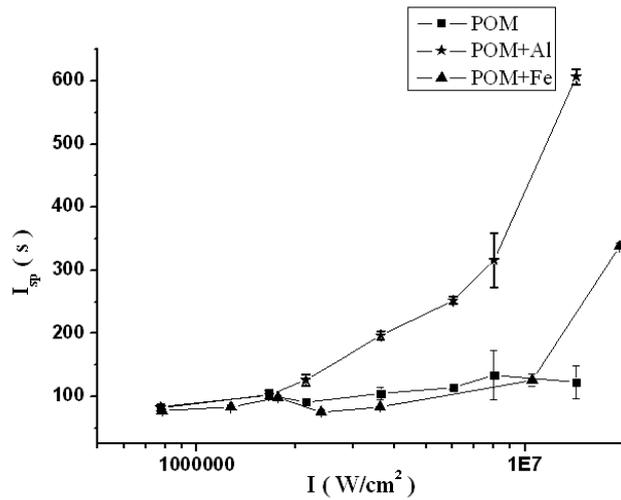
Figure 5. Experimental  $I_{sp}$  versus laser power density curves for three kinds of propellants
