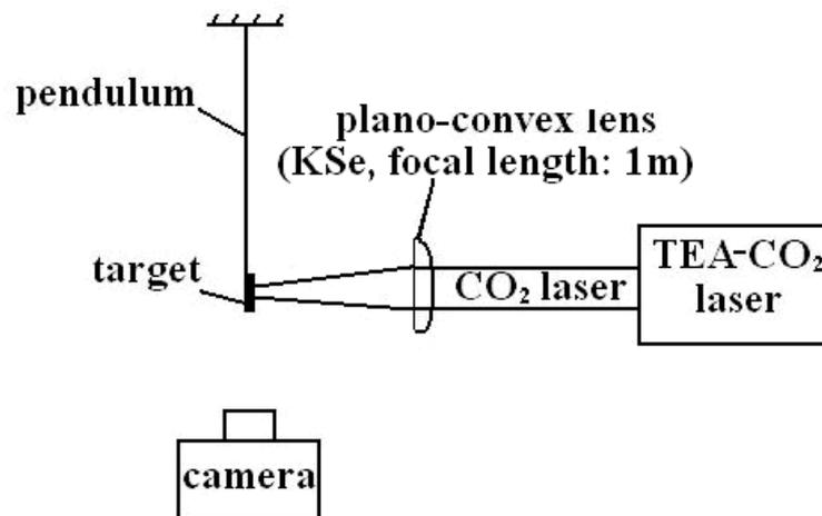
Figure 2. Schematic for the propulsion performance experiment
