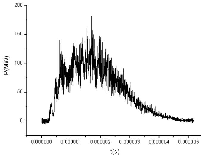
Figure 7. The laser pulse waveform in confirmatory experiments
