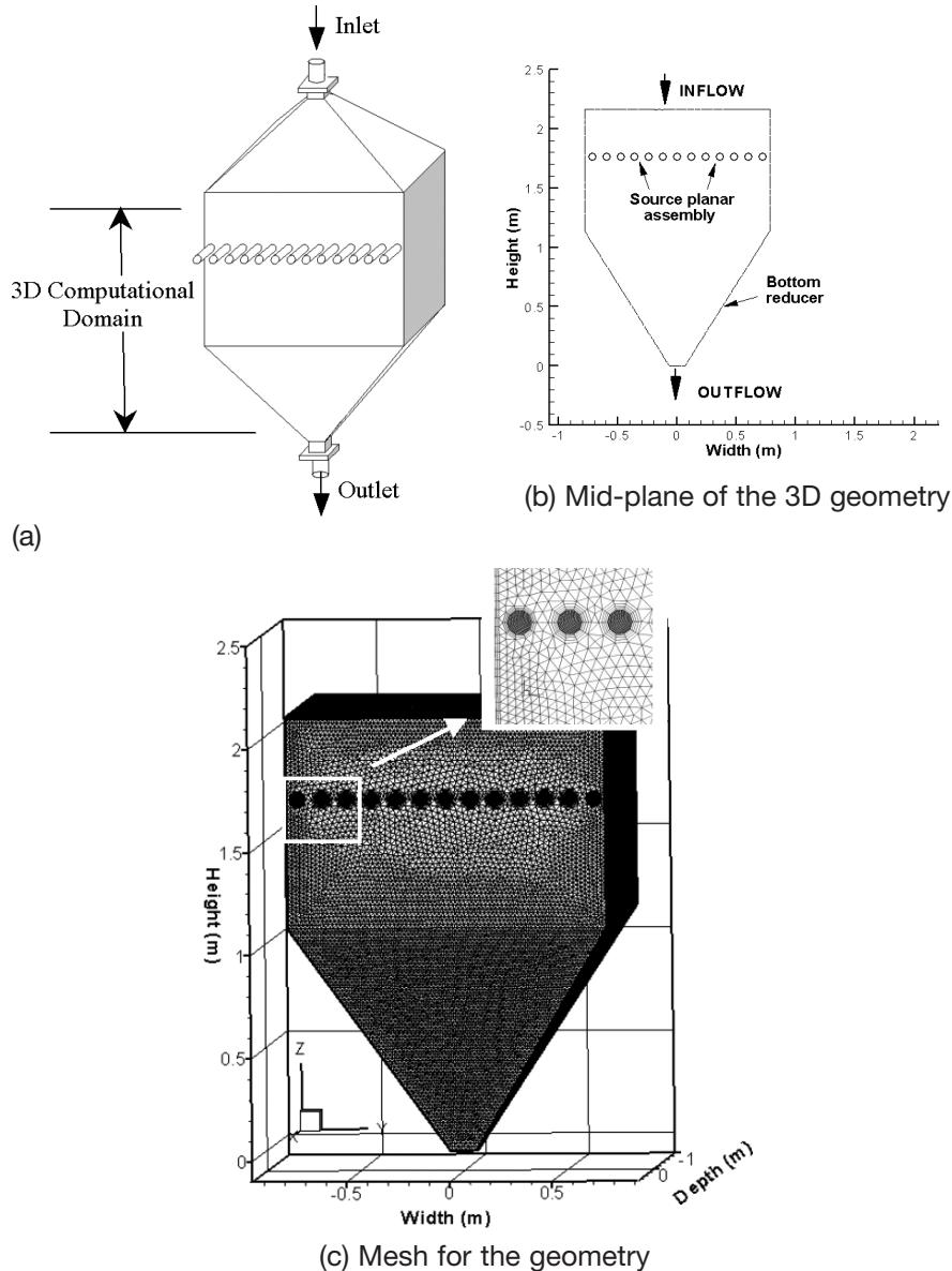
Figure 2. (a) Existing irradiation vessel geometry, (b) Mid-plane illustrating the gamma source planar assembly and (c) Mesh for the geometry in SHRI.
