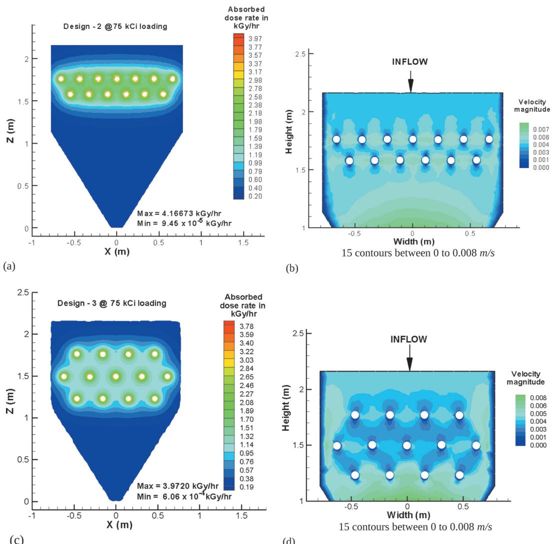
Figure 9. Estimated absorbed dose rate for (a) design-2, (c) design-3, (e) design-4 and time mean velocity magnitude for (b) design-2, (d) design-3, (f) design-4
