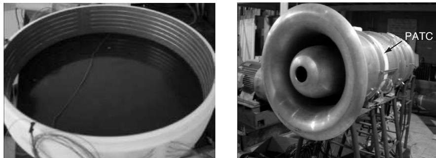
Figure 30. Plasma actuation treated casing and its application on a compressor.
