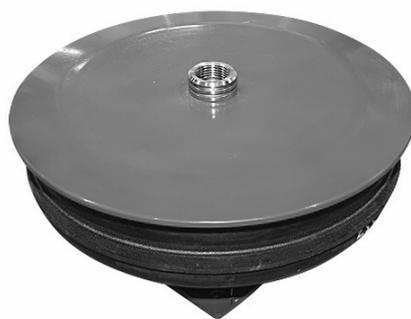
*The old technology or steel coil springs used in the suspension of Indian Railways coaches is now being replaced with Trelleborg’s rubber components or air spring – a rubber mounting combined with rubber bellows, which improves secondary suspension, resulting in a smooth and comfortable journey for passengers. Photo Trelleborg*
