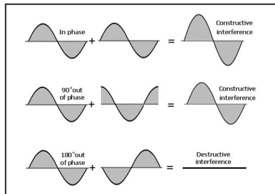
Figure1. *Constructive and destructive interferences occurring in the third case in the wave phases of two sources*
