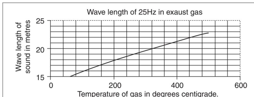
Figure 5 Wavelength of 25Hz in exhaust gas
