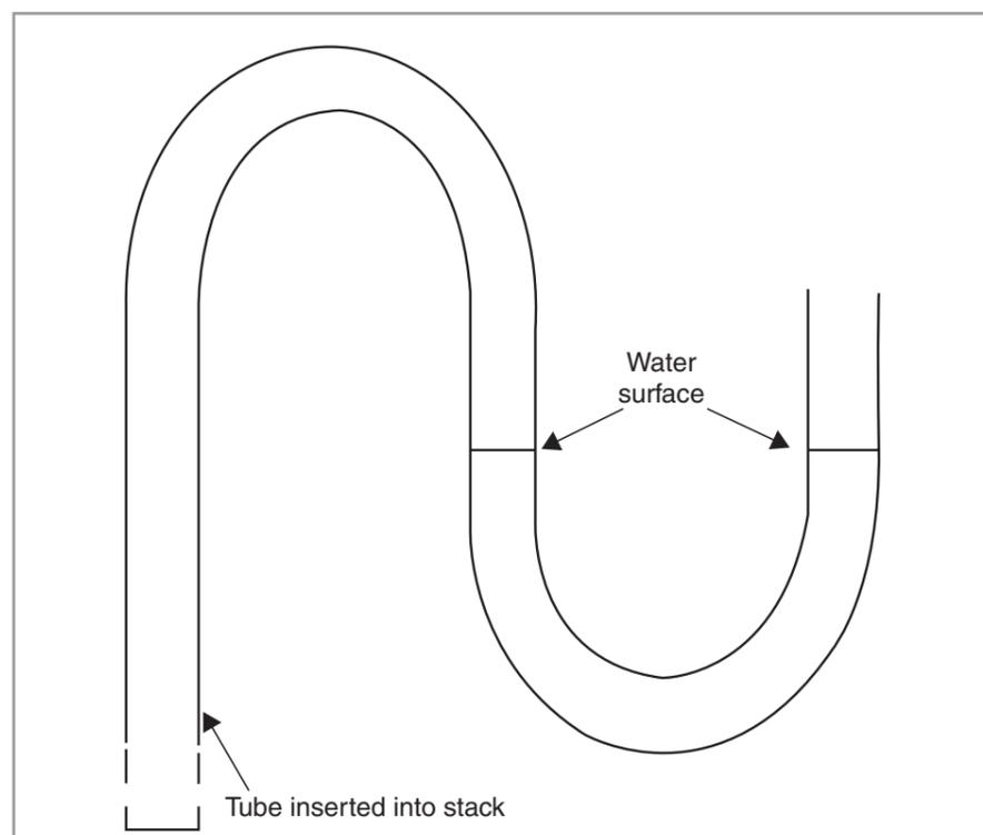
Figure 6 Manometer for location of pressure maximum
