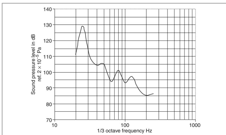
Figure 4 *Noise 10m from exhaust stack*
