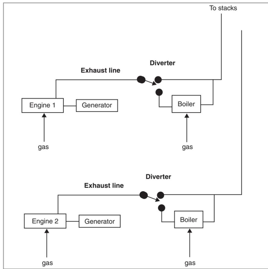
Figure 1 Arrangement of boiler room
