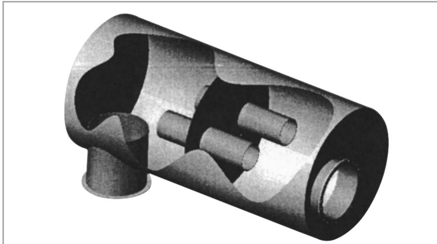
Figure 10 Reactive exhaust silencer fitted close to each engine
