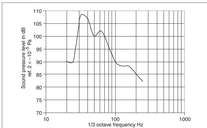
Figure 3 *Spectrum near to boiler No.2*
