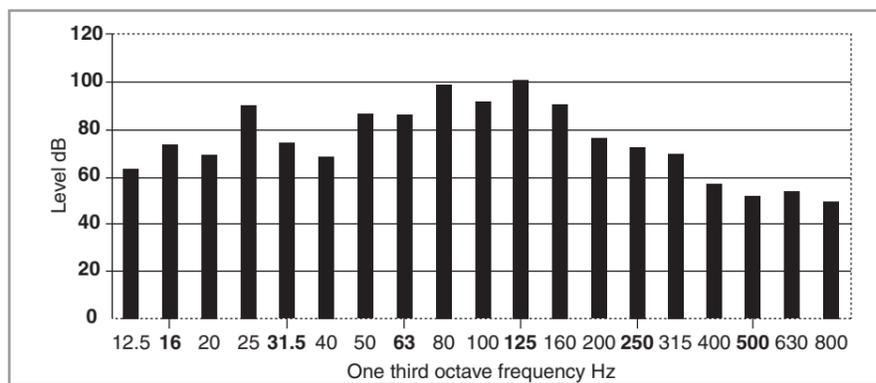
Figure 7 Conventional 1/3 octave analysis of the engine noise near the top of the stack
