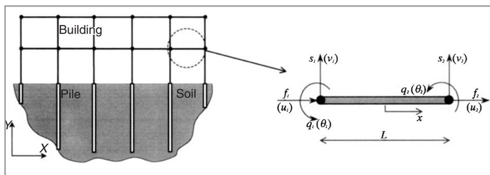
Figure 1 A typical DSM element from a two-dimensional portal frame. The generalised forces  $f$ ,  $s$  and  $q$ , and the corresponding generalised displacements ( $u$ ,  $v$  and  $\theta$ ) are related through the element's dynamic-stiffness matrix. Junctions between elements are known as nodes ( $\bullet$ ).
