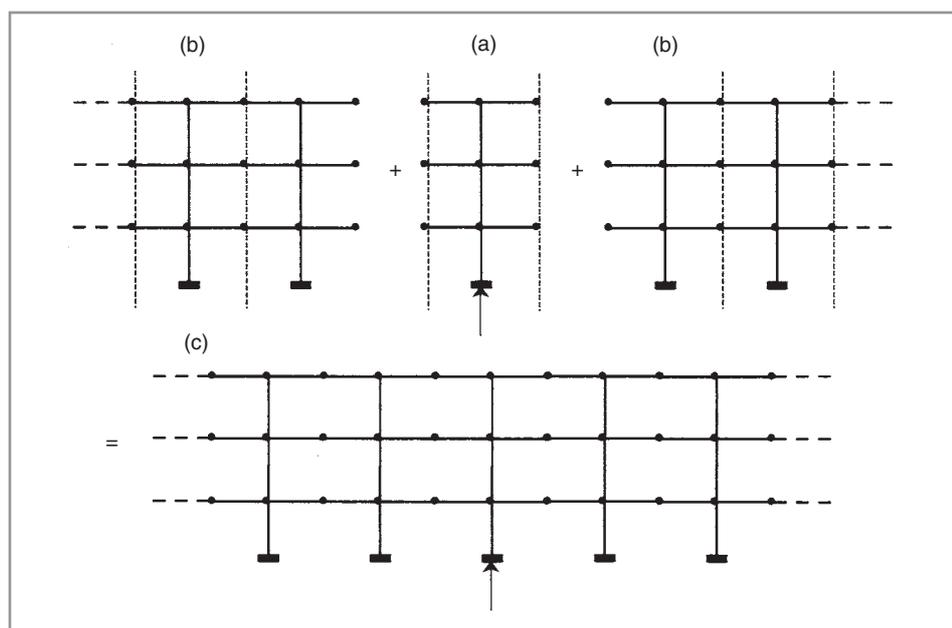
Figure 2 An infinitely long two-dimensional portal-frame model of a building, based on the dynamic-stiffness method and periodic structure theory. The central loaded unit (a) is coupled to two semi-infinite structures (b) to form the complete model (c). The repeating units are defined by dashed vertical lines.
