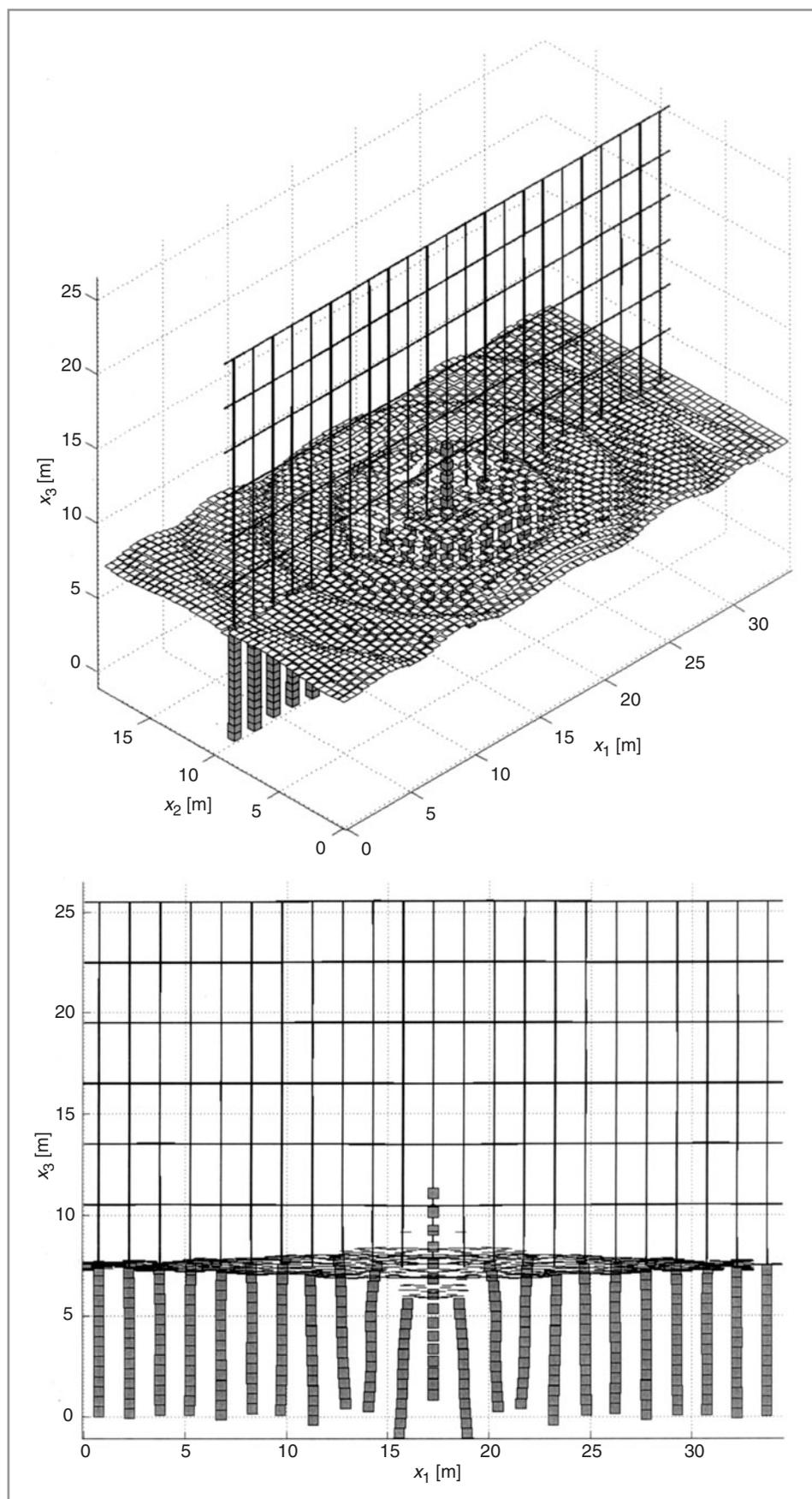
Figure 8 *Vibration of a '5 Hz' base-isolated hospital as predicted by the generic model. The 50 Hz excitation corresponds to a vertical unit-amplitude force applied to the central pile-head prior to the construction of the building. All displacements are magnified by  $1 \times 10^{10}$ .*
