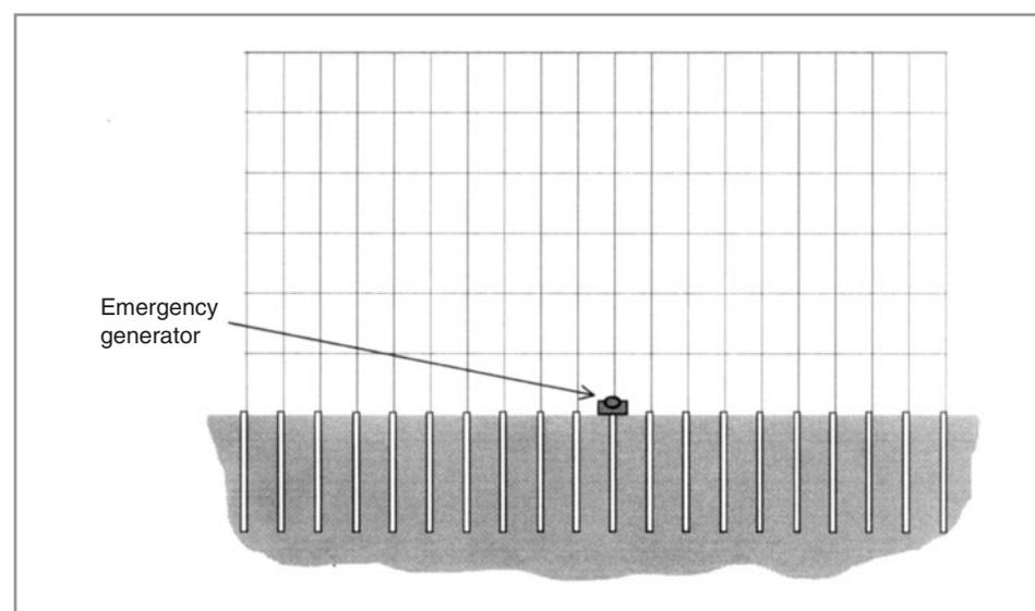
Figure 6 Schematic elevation of a new hospital. An emergency generator located at ground-floor level may lead to excessive levels of internal vibration and base isolation of the building is a potential solution
