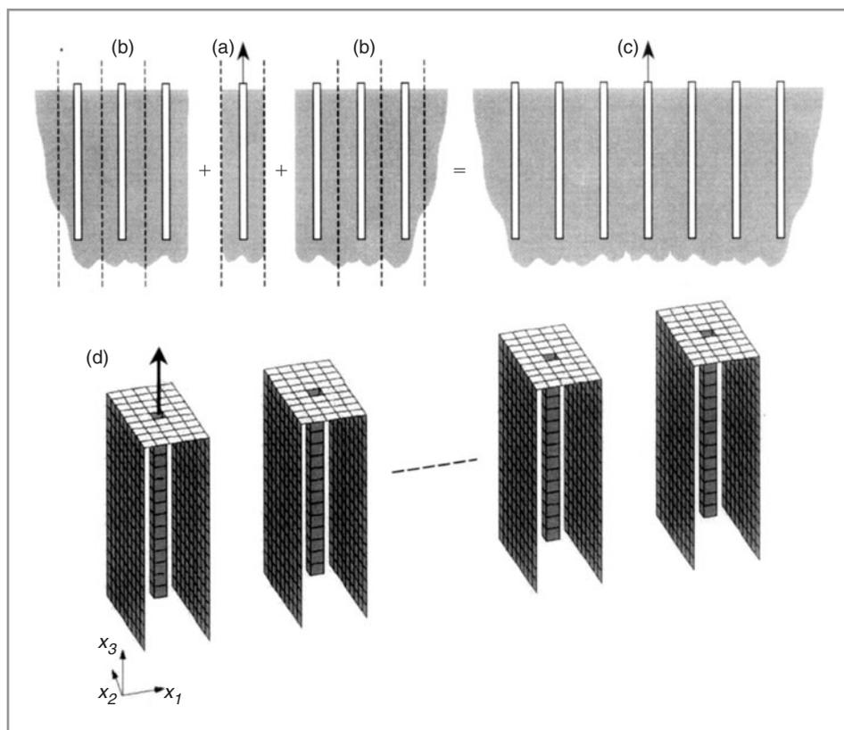
Figure 4 An infinitely long three-dimensional model of a piled foundation, based on the boundary-element method and periodic structure theory. The central loaded unit (a) is coupled to two semi-infinite models (b) to form the complete model (c). The BEM mesh for the soil component of one half of the model is also shown (d).
