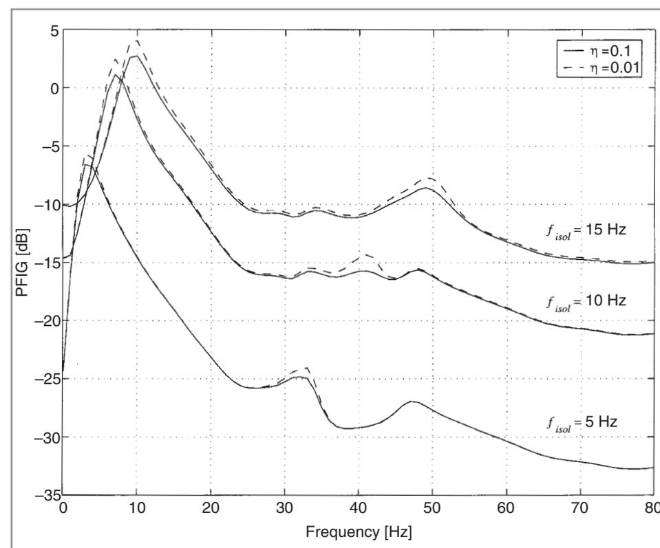
Figure 9 Variation with frequency in the power-flow insertion gain of a base-isolated hospital, as predicted by the generic model. Isolation frequencies of 5, 10 and 15 Hz are considered, provided by bearings with internal damping loss factors of 0.1 and 0.01. The excitation corresponds to a vertical unit-amplitude force applied to the central pile-head prior to the construction of the building.
