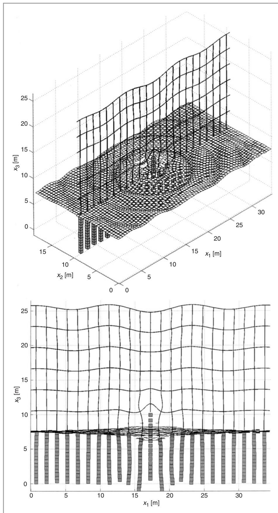
Figure 7 *Vibration of an unisolated hospital as predicted by the generic model. The 50 Hz excitation corresponds to a vertical unit-amplitude force applied to the central pile-head prior to the construction of the building. All displacements are magnified by  $1 \times 10^{10}$ .*
