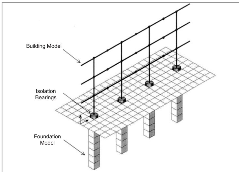
Figure 5 Schematic isometric projection of the generic model. The infinitely long two-dimensional portal-frame model of a building is coupled to the infinitely long three-dimensional model of a piled foundation.
