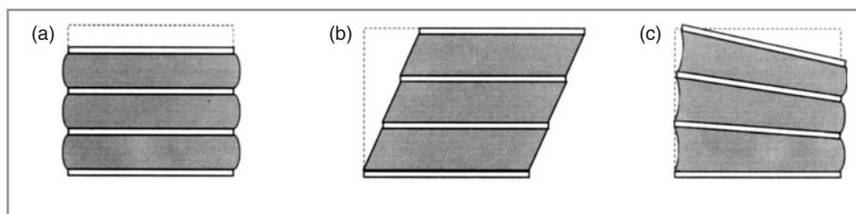
Figure 3 The three modes of deformation associated with an isolation bearing are described by three stiffnesses: (a)  $k_v$  vertical compression; (b)  $k_h$  horizontal shear; and (c)  $k_q$  rotation.
