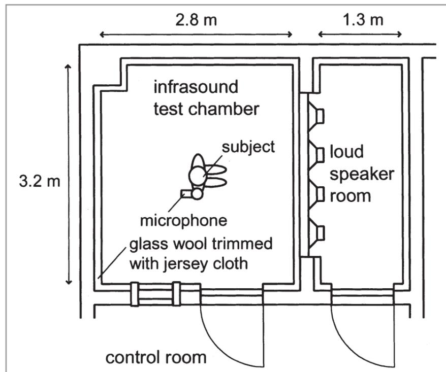
Figure 1. Schematic diagram of the plan of the experimental facilities used in this study
