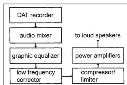
Figure 2. Sound generation system used in the experiment
