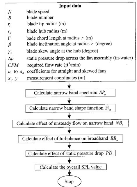
Figure 1. Flow chart for calculating noise spectrum of an engine cooling fan assembly
