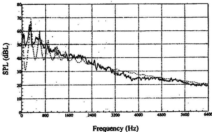
Figure 12. Comparison of noise spectra from Type B fan with shroud/radiator/condenser running in the high-speed regime. Solid line: Measured; Dashed line: Calculated.
