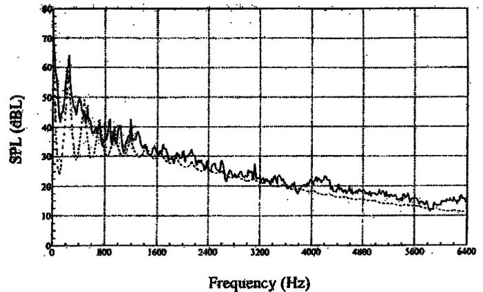
Figure 4. Comparison of noise spectra from Type A fan with shroud running in the low-speed regime. Solid line: Measured; Dashed line: Calculated.
