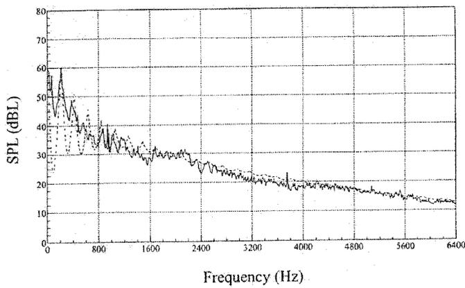
Figure 9. Comparison of noise spectra from Type B fan with shroud running in the low-regime. Solid line: Measured; Dashed line: Calculated.
