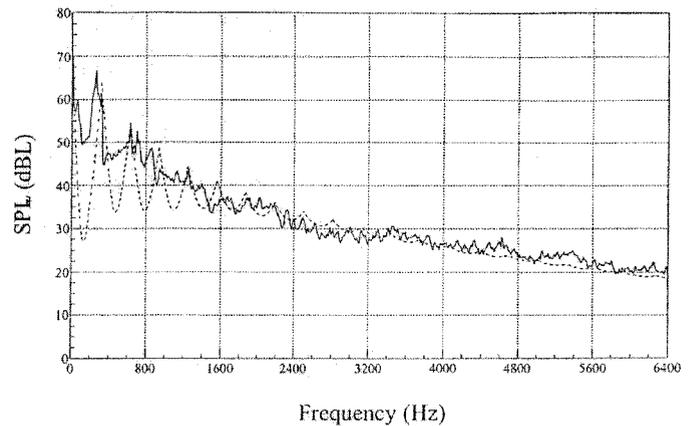
Figure 7. Comparison of noise spectra from Type A fan with shroud/radiator/condenser running in the high-speed regime. Solid line: Measured; Dashed line: Calculated.
