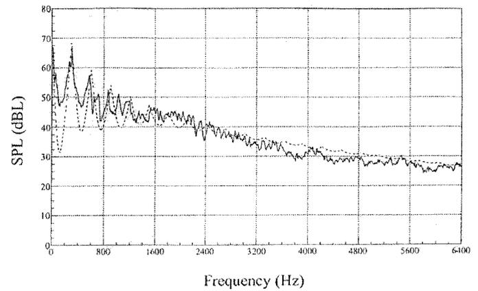
Figure 10. Comparison of noise spectra from Type B fan with shroud running in the high-speed regime. Solid line: Measured; Dashed line: Calculated.
