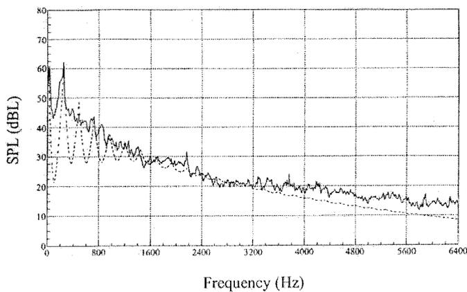
Figure 6. Comparison of noise spectra from Type A fan with shroud/radiator/condenser running in the low-speed regime. Solid line: Measured; Dashed line: Calculated.
