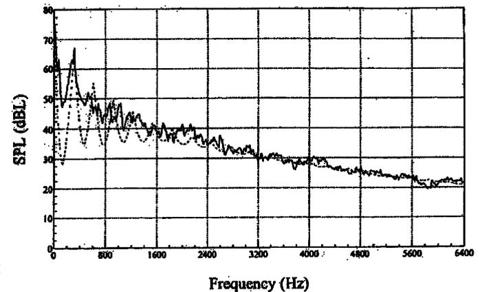
Figure 5: Comparison of noise spectra from Type A fan with shroud running in the high-speed regime. Solid line: Measured; Dashed line: Calculated.
