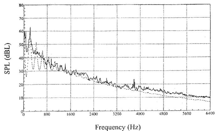
Figure 11. Comparison of noise spectra from Type B fan with shroud/radiator/condenser running in the low-speed regime. Solid line: Measured; Dashed line: Calculated.
