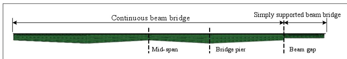
Figure 4 Analysis positions on the bridge
