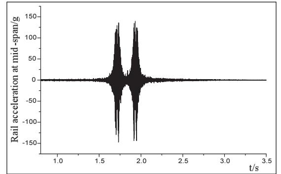
Figure 6. Acceleration-time curve of damping rail
