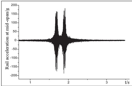
Figure 5. Acceleration-time curve of standard rail
