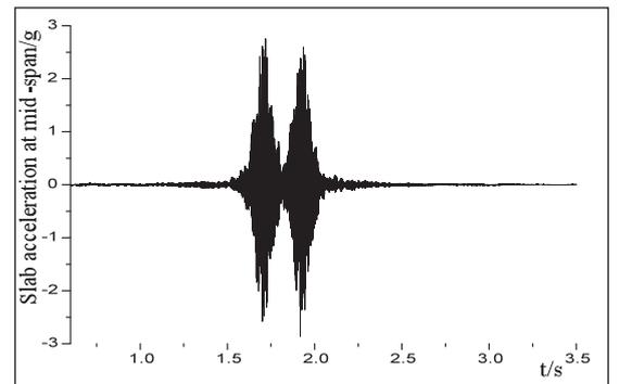
Figure 8. Acceleration-time curve of track slab with damping rail
