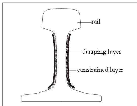
Figure 1. *Constrained damping rail*
