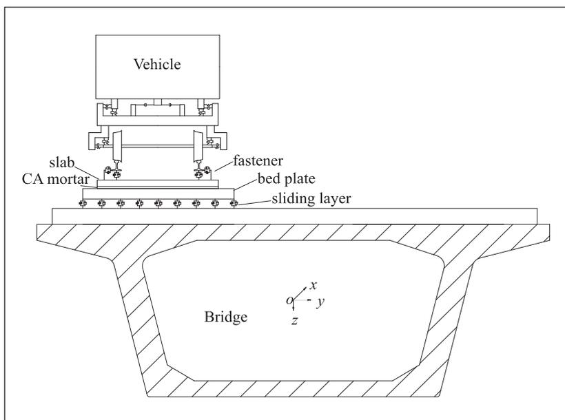
Figure 2. *Vehicle-ballastless slab track-bridge mechanical model*
