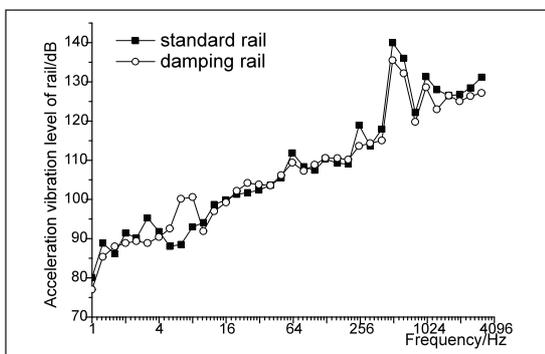
Figure 11. Acceleration vibration level of standard rail and damping rail at bridge mid-span
