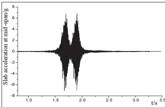
Figure 7. Acceleration-time curve of track slab with standard rail
