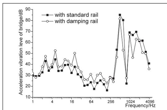
Figure 13. Acceleration vibration level of bridge with and without damping rail at bridge mid-span
