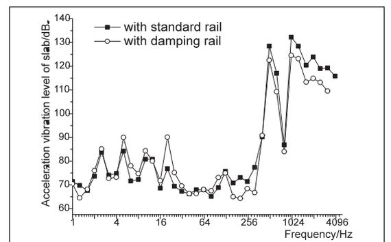
Figure 12. Acceleration vibration level of track slab with and without damping rail at bridge mid-span
