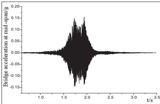
Figure 9. Acceleration-time curve of bridge with standard rail
