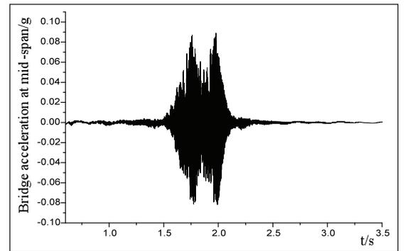
Figure 10. Acceleration-time curves of bridge with damping rail
