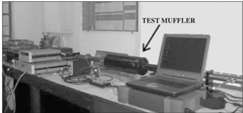
Figure 13. Transmission loss testing setup for muffler [17]
