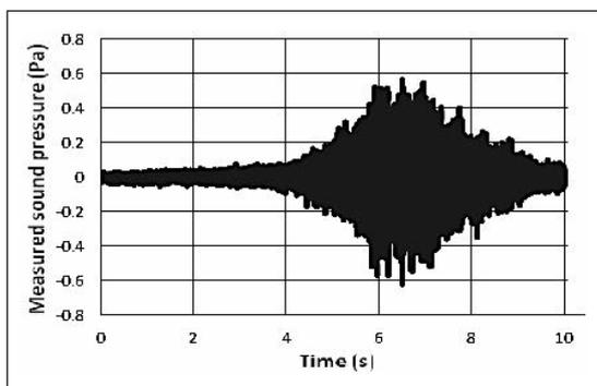
Figure 5. Measured sound pressure time waveform during a passby noise test
