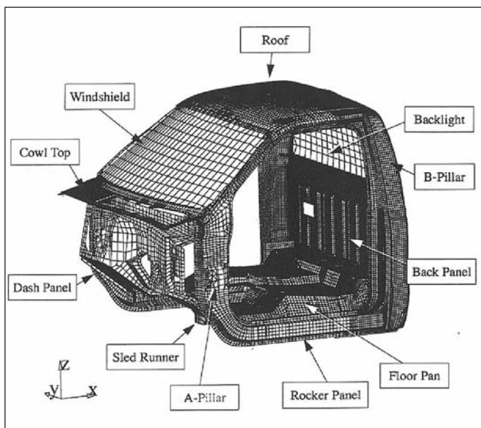
Figure 1. FE model of a truck cab [4]
