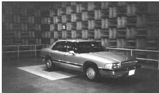
Figure 9. *Hemi-anechoic chamber used for automobile noise measurements [16]*
