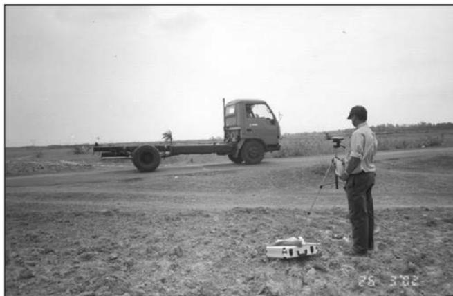
Figure 4. Passby noise measurements of a truck at a test track
