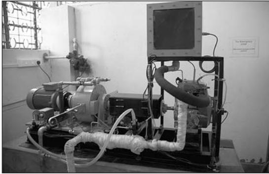
Figure 11. Instrumented engine-eddy current dynamometer test rig
