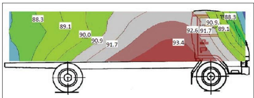
Figure 7: Radiated noise map of a truck
