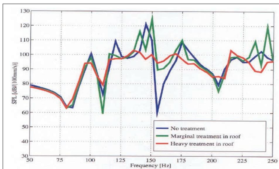
Figure 2. CAE prediction of SPL at DRE with various sound absorbing materials [4]
