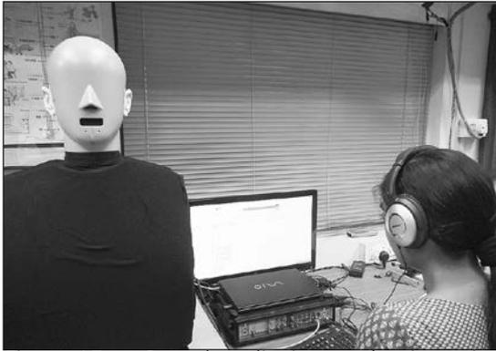
Figure 15. Sound quality jury evaluation using HATS in the laboratory
