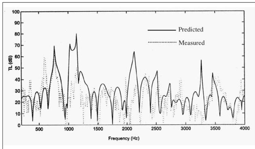
Figure 14. Measured and predicted transmission loss of the muffler [17].
