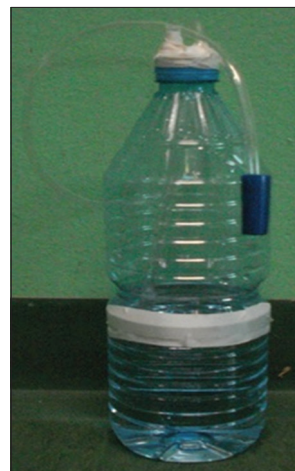
Figure 1: Improvised underwater seal apparatus
