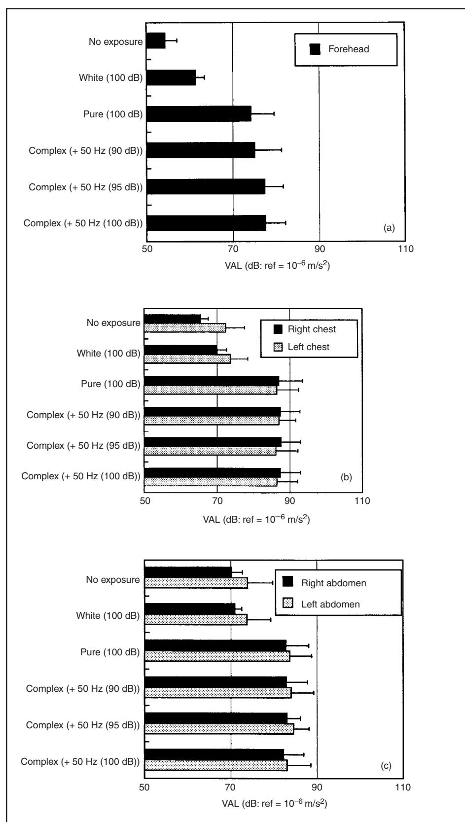
Figure 3 The vibration acceleration levels (means  $\pm$  SD) of the 31.5-Hz component in the noise-induced vibration measured for no noise stimulus, the white noise stimulus, the 31.5-Hz pure tonal stimulus, and the three complex noise stimuli in which the 31.5-Hz noise component was set at 100 dB(SPL). They were measured (a) at the forehead, (b) at the chest, and (c) at the abdomen.
