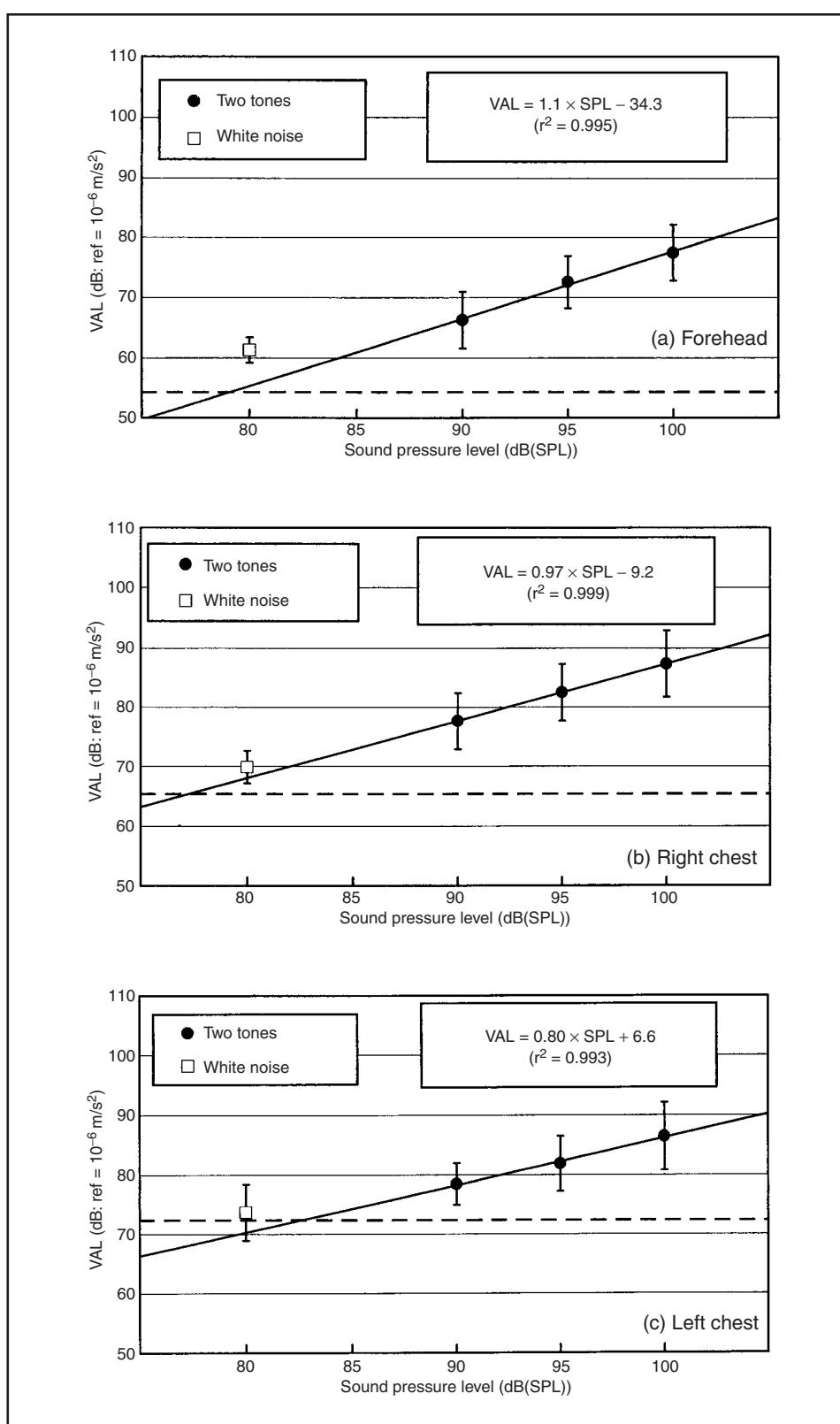
Figure 5 The vibration acceleration levels (means  $\pm$  SD) of the 31.5-Hz component in the noise-induced vibration measured for the three complex noise stimuli in which the 50-Hz noise component was set at 100 dB(SPL). They (black circles) were measured (a) at the forehead, (b) at the right chest, (c) at the left chest, (d) at the right abdomen, and (e) at the left abdomen. Please refer to the Results section for more details
