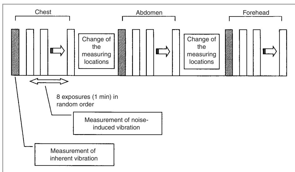
*Figure 2 The procedure of the measurement In the first session, noise-induced vibrations were measured at the chest. In the second and last sessions, noise-induced vibrations were measured at the abdomen and at the forehead, in that order.*
