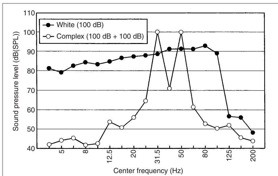
*Figure 1 An example of the frequency spectra of the noise stimuli. The spectra shown are for the white noise stimulus and for the complex noise stimulus composed of a 31.5-Hz, 100-dB tone and a 50-Hz, 100-dB tone. These were measured at the center of the test chamber (120cm in height).*
