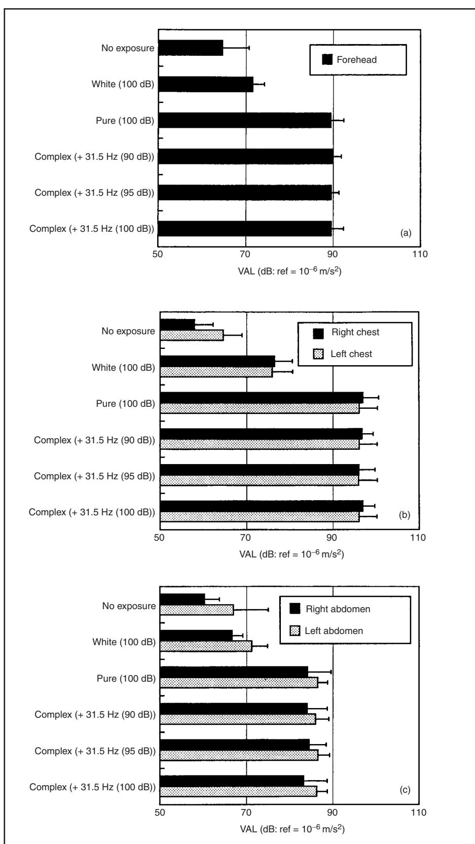
**Figure 4** The vibration acceleration levels (means  $\pm$  SD) of the 50-Hz vibration measured for no noise stimulus, the 50-Hz pure tonal stimulus, and the three complex noise stimuli in which the 50-Hz noise component was set at 100 dB(SPL). They were measured (a) at the forehead, (b) at the chest, and (c) at the abdomen.
