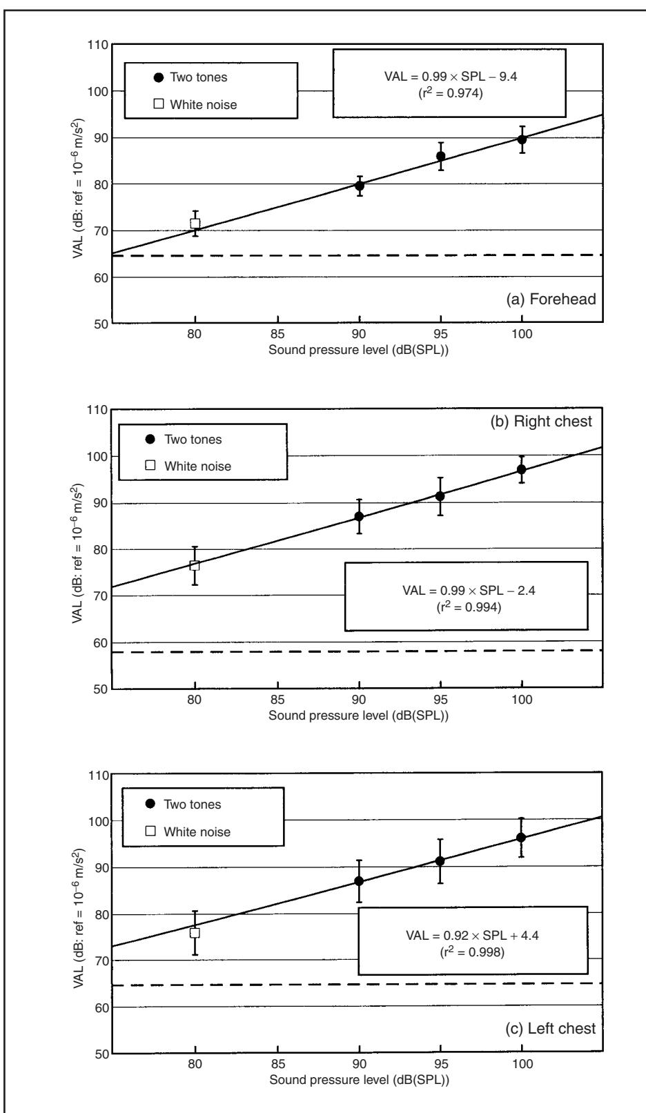
Figure 6 The vibration acceleration levels (means  $\pm$  SD) of the 50-Hz component in the noise-induced vibration measured for the three complex noise stimuli in which the 31.5-Hz noise component was set at 100 dB(SPL). They (black circles) were measured (a) at the forehead, (b) at the right chest, (c) at the left chest, (d) at the right abdomen, and (e) at the left abdomen. Please refer to the Results section for more details.
