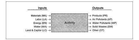
Figure 3. Inputs and outputs associated with an activity.
